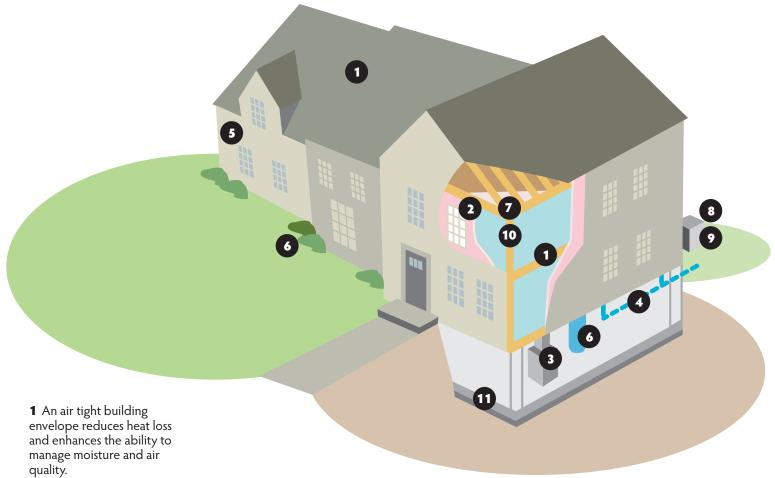
2 Thermal performance: Superior insulation systems and Low-E Argon double glazed windows reduce the energy required to keep a
